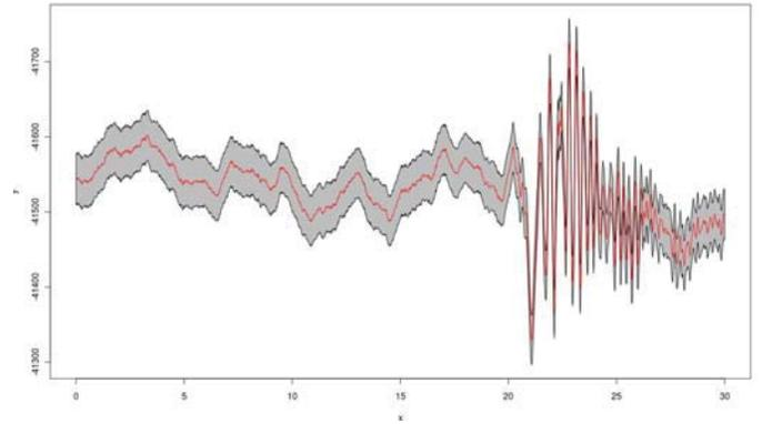
Fig. 2. Longitudinal movement of a GPS receiver located in Japan, during the Tōhoku earthquake. The read line is the reading and the gray area is one standard deviation border around the reading.
